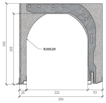
Option brackets and ligatures [PDF]: in accordance with the technical advice of the CSTB, the reinforced boxes will be ligatures to the chain and fixed to the upper crosspiece using brackets. Brackets and ligatures are available separetely or integrated into the box during production.
