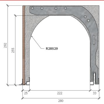
Option brackets and ligatures [PDF]: in accordance with the technical advice of the CSTB, the reinforced boxes will be ligatures to the chain and fixed to the upper crosspiece using brackets. Brackets and ligatures are available separetely or integrated into the box during production.
